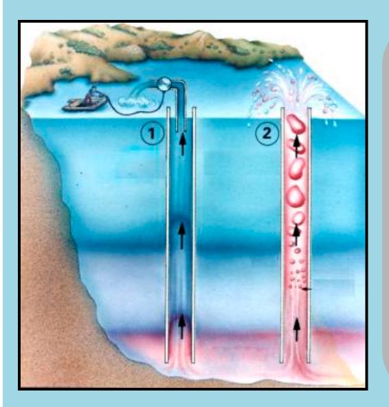
Degassing columns were installed at Lake Nyos to prevent a similar disaster.
